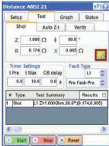
Distance relay test setup
