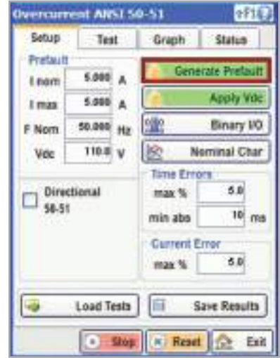
Over-current relay test result
